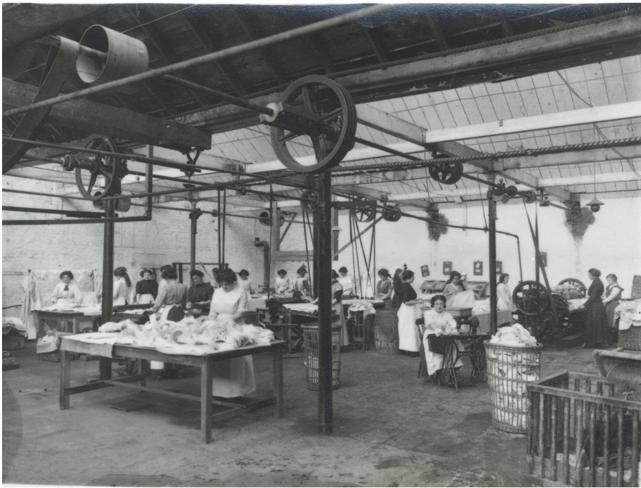
The Smoothing Room, Armagh City Steam Laundry c1915. Note the large gas heated calendar on the right which smoothed large items such as sheets and the table of shirt collars (centre) being smoothed and sorted.
